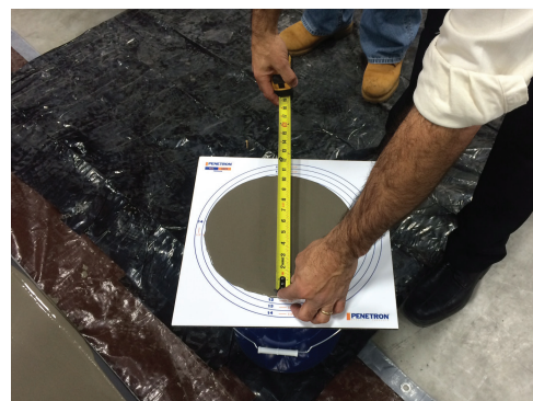
Measuring the Fail-Safe board to check material viscosity.
